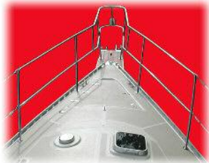
Extended stainless steel bow pulpit makes it safer to be on the foredeck.
