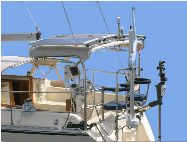
Charging power can be supplied by solar panels, wind genera-
