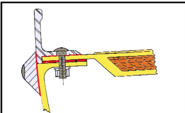
The four-way deck-bonding system, an example of a belt and suspender system which makes the Caliber 40LRC so rugged.
