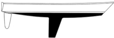
High performance fin keel is fast, but at the expense of directional stability. Hull shape creates a quick, uncomfortable motion offshore with limited load carrying capacity.
