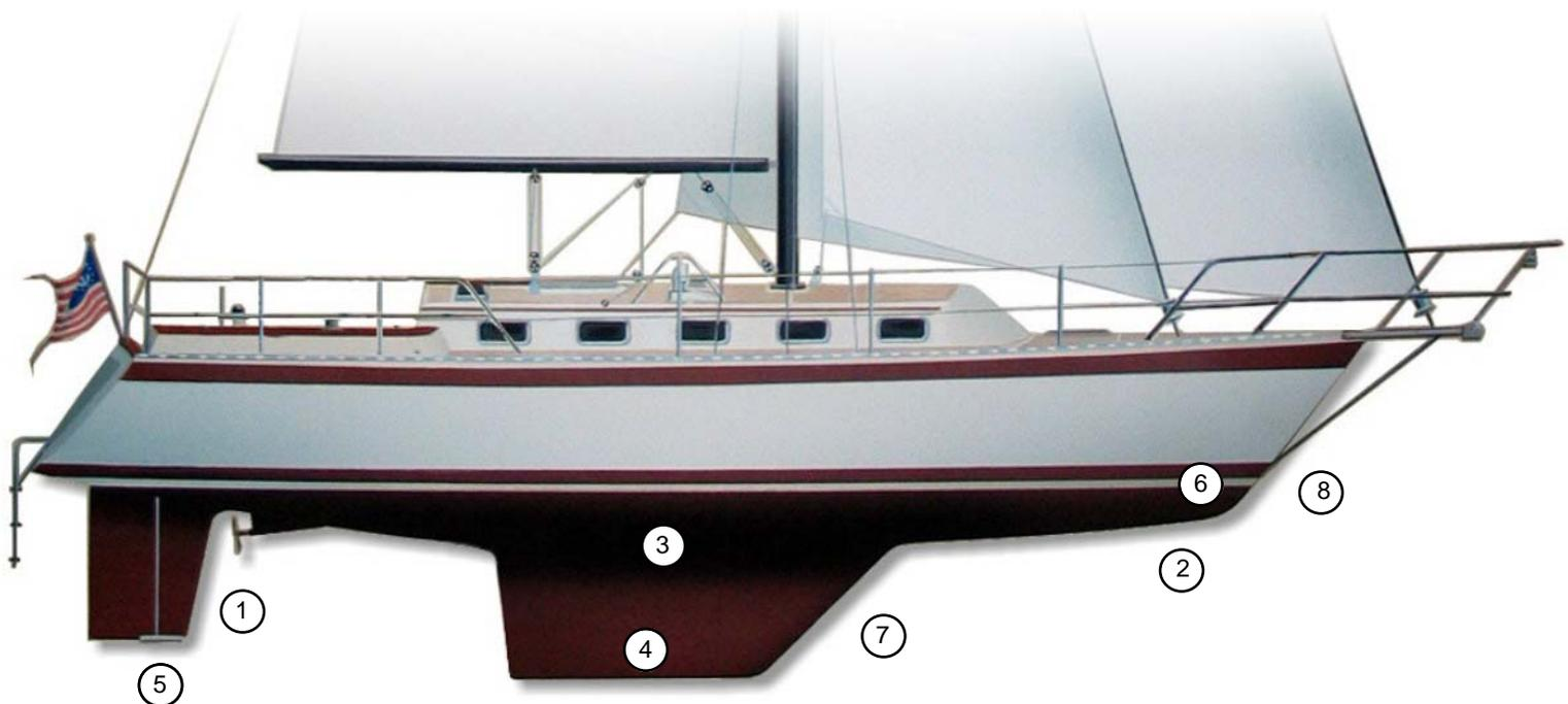
1. Skeg/Rudder combination designed to maximize both maneuverability and strength.
