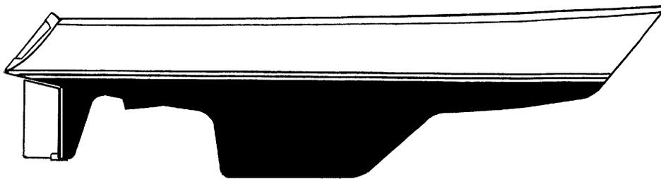
Proven combination of the two extreme types creates a hull that have these characteristics: high pointing ability, excellent directional stability, easy tacking (light wind), and high mobility during docking situations.
