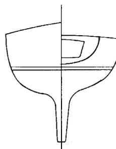
**Moderate displacement, moderate draft and moderate beam. A safe, comfortable, offshore cruising type hull design.**
